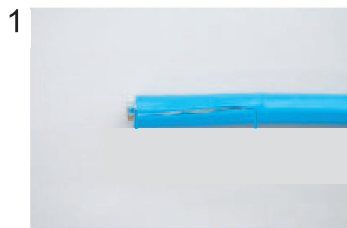
1 Expose inner vinyl sheath.
