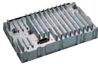
Power Amplifier Module of the Solid-State transceiver
