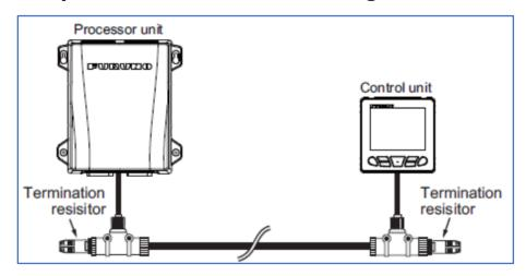
**Does the NavPilot 300 require a control head?** Upon introduction of the NavPilot 300 a control head will be required. However, full control from a TZT2 MFD is planned with version 6.1 software. At that time, it should be possible to operate without any control head in the system. TZT2 version 6.1 software is expected to be available Fall 2018.
