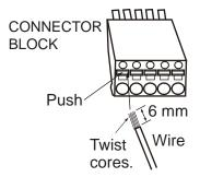
How to put wire into connector block
