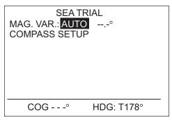
With a magnetic heading sensor (PG-500/700 etc.), magnetic variation information is necessary to display true heading data. In almost all cases, a GPS will be connected to the NAVpilot and the GPS will send this variation information to the NAVpilot automatically. Therefore, select "AUTO". In special cases where a manual variation is required, you may input these values manually. Note that this selection is only effective when the heading indication for the NAVpilot is selected to "TRUE".
