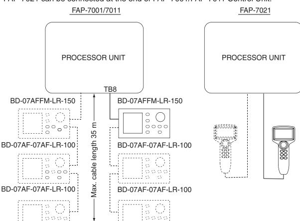
• FAP-7021 can be connected at the end of FAP-7001/FAP-7011 Control Unit.
