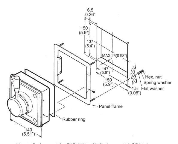
How to flush mount the FAP-6221 with flush mount kit OP64-4
