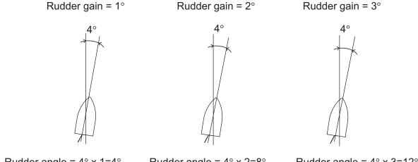
Rudder angle =  $4^{\circ}$  x  $1=4^{\circ}$
