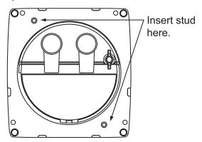
3. Set the unit to the mounting hole. Fasten the unit with the flat washers, spring washers and wing nuts (supplied).
