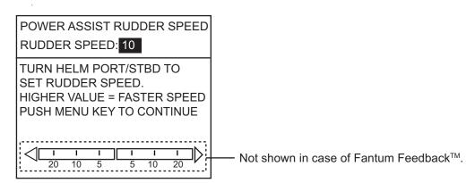
7. Turn the helm to port and starboard to set [POWER ASSIST RUDDER SPEED], and then push the knob. The higher the setting, the stronger the power assist.
