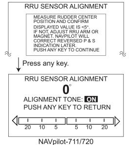
5. With the rudder physically centered, confirm that the displayed rudder angle indication is less than or equal to ±5°. If not, you must adjust the rudder sensor body or magnet position (for Teleflex linear sensor AR4502) so that the indicator is within ±5° before continuing.
