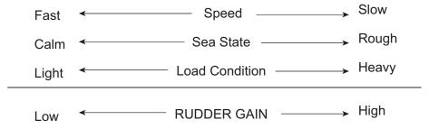
[COUNT RUDDER]: If the boat is heavily loaded, the heading could change excessively because of inertia. This phenomenon causes the vessel to "overshoot" the intended course. If this happens, the NAVpilot will steer the rudder to the opposite side and the heading will turn in opposite direction excessively again. In an extreme case the heading oscillates several times until it finally settles in the new course. An adjustment known as "counter rudder" prevents this kind of oscillation.
