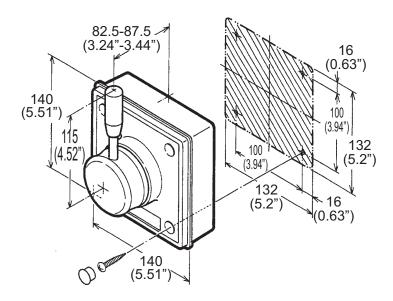
To mount the FAP-6221/6212 in a panel, the optional flush mount kit OP64-4 or OP64-5 is required.
