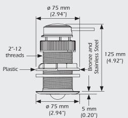
Airmar's innovative housing design incorporates a self-closing valve to minimize water flow into boat when the insert is removed.
