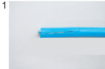
Expose inner vinyl sheath.
