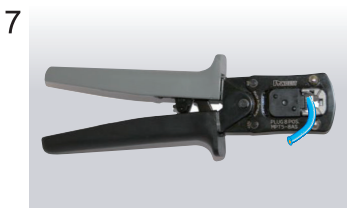
Using special crimping tool MPT5-8AS (PANDUIT CORP.), crimp the modular plug. Finally, check the plug visually.
