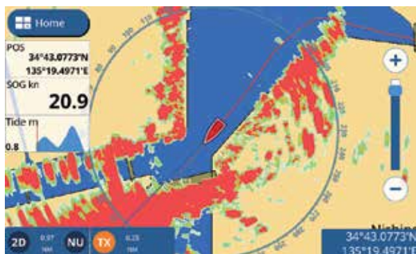
Mode superposition radar
