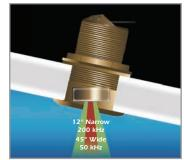
The ceramic element is tilted inside the housing, which compensates for your boats deadrise. This aims the beam straight toward the bottom, resulting in stronger echo returns and more accurate depth readings.
