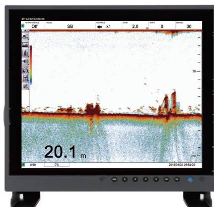
Main monitor: Echoes from FCV-38 fish finder displayed.
