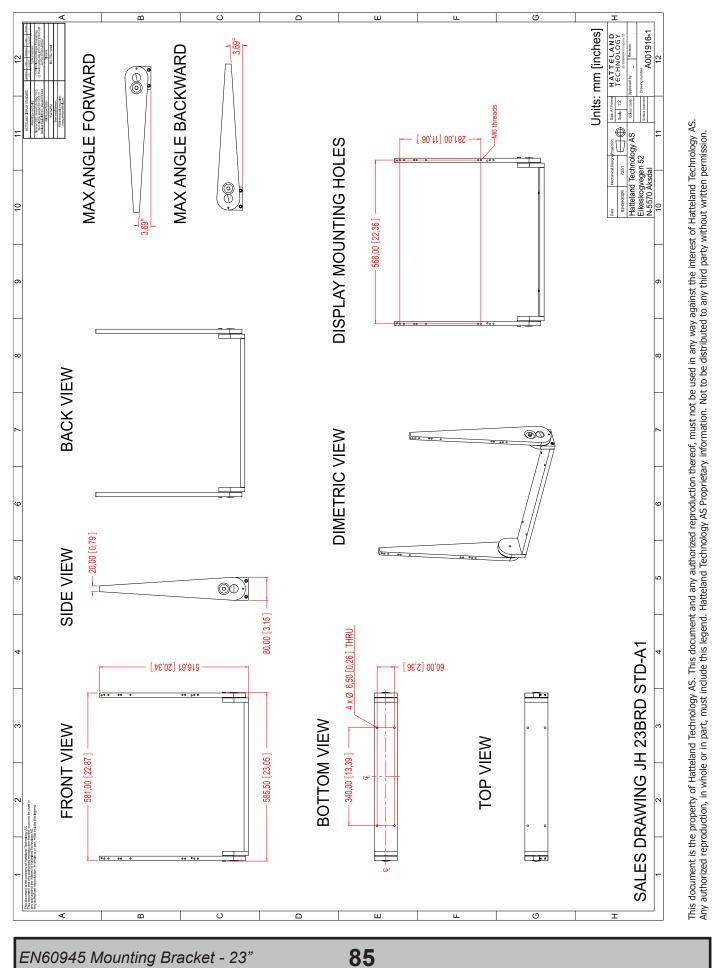
Dimensions might be shown with or without decimals and indicated as mm [inches]. Tolerance on drawings is +/- 1mm. For accurate measurements, check relevant DWG file.
