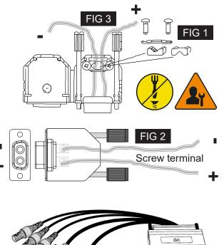
The cable could also be customized upon customer request for length or to support other signal types and connectors. Using any other cable/housing design to connect to the display units could result in severe damage to components!
